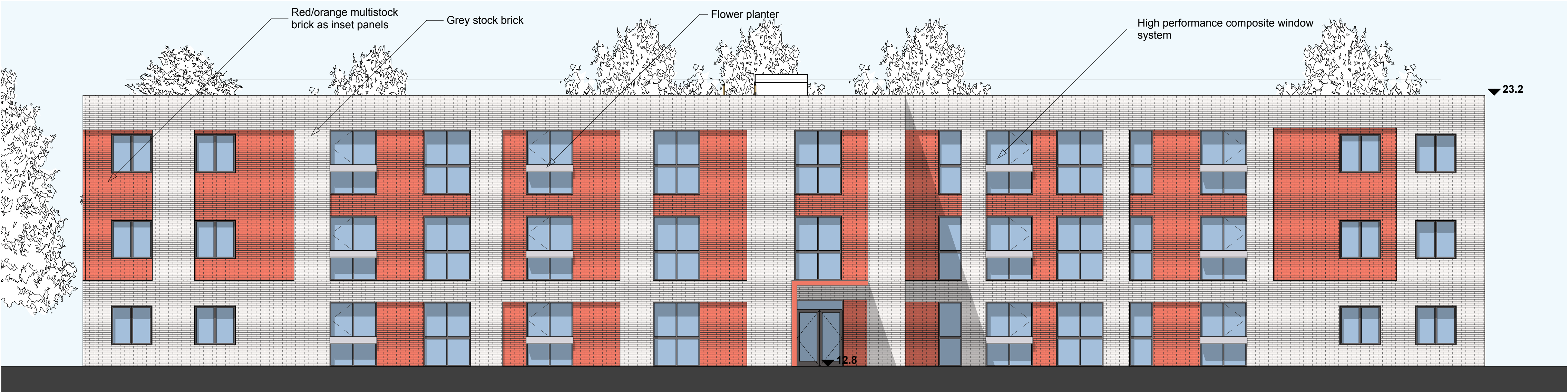
329 Supported Living South - West Elevation 1:100
