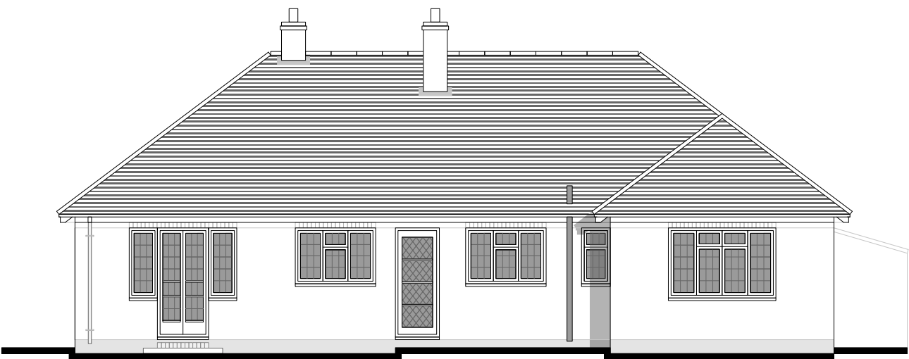
Existing Rear Elevation at 1:100 scale SOUTH EAST
