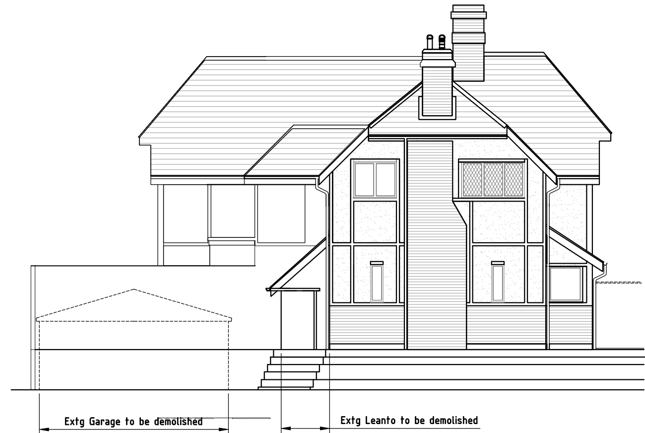
Existing North Elevation
