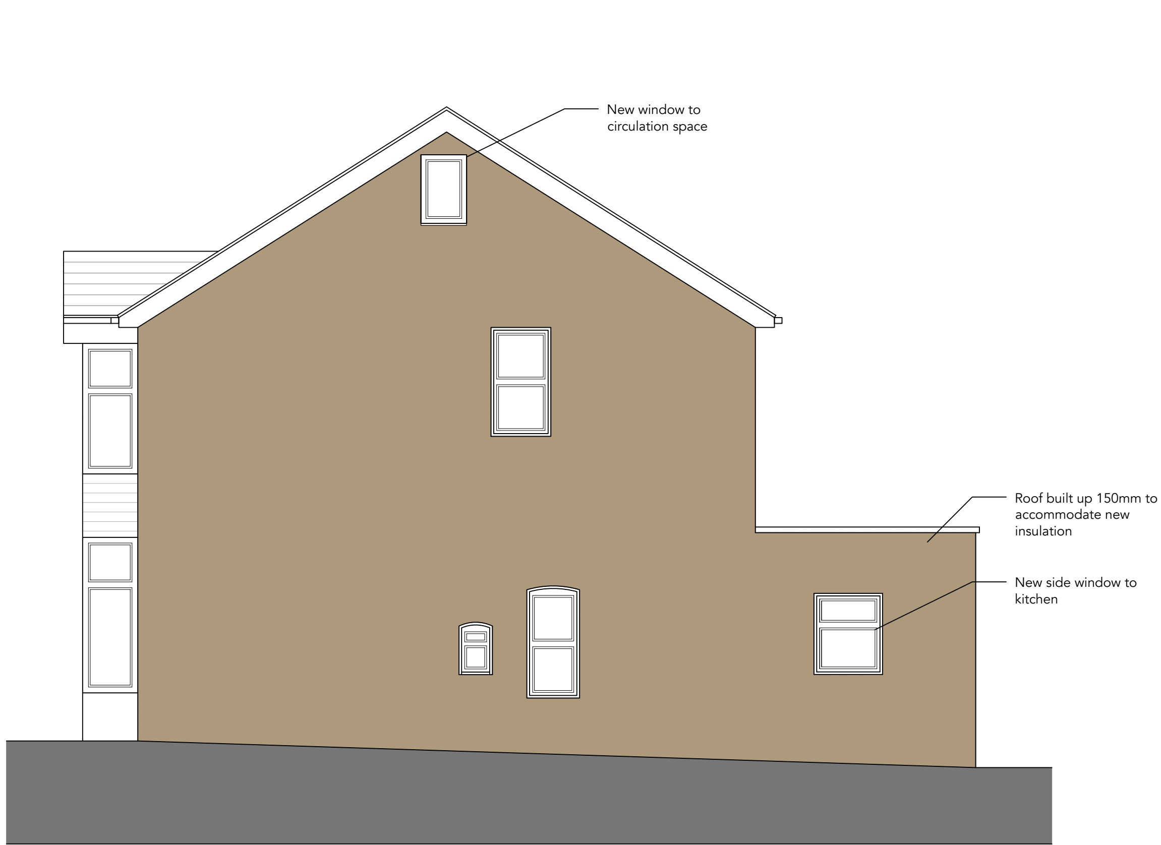
2 PROPOSED SOUTH-EAST / SIDE ELEVATION Scale: 1:50
