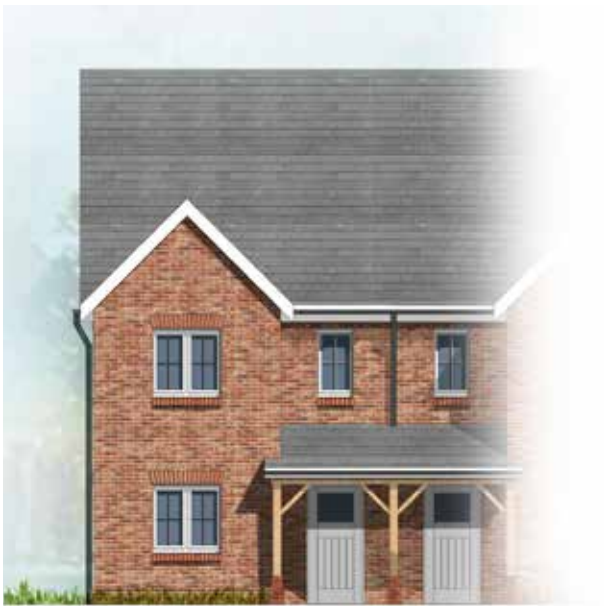
TYPE 2 Red multi brick Mid slate roof tile White UPVC casement windows with glazing bars Brick jack headers & sills Timber framed entrance canopy on posts Chimneys to selected plots
