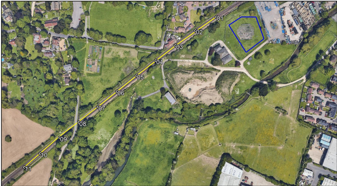
Figure 12 Section of railway line where solar reflections are geometrically possible (yellow line) – aerial image
