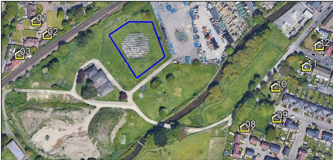
Figure 9 Dwellings towards which solar reflections are geometrically possible – aerial image
