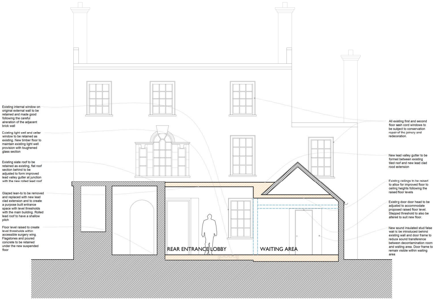
Proposed Section CC 1:100 at A3
