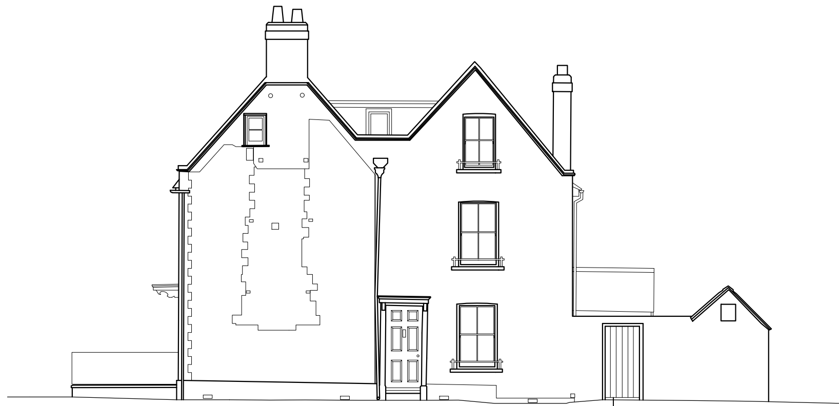
SOUTH WEST ELEVATION 1:100
