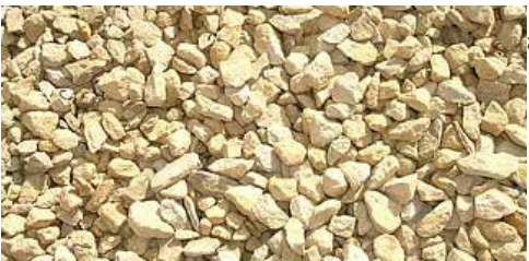
10mm Gravel to parking area for parking and turning areas
