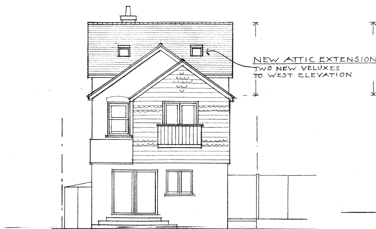
WEST FACING ELEVATION
