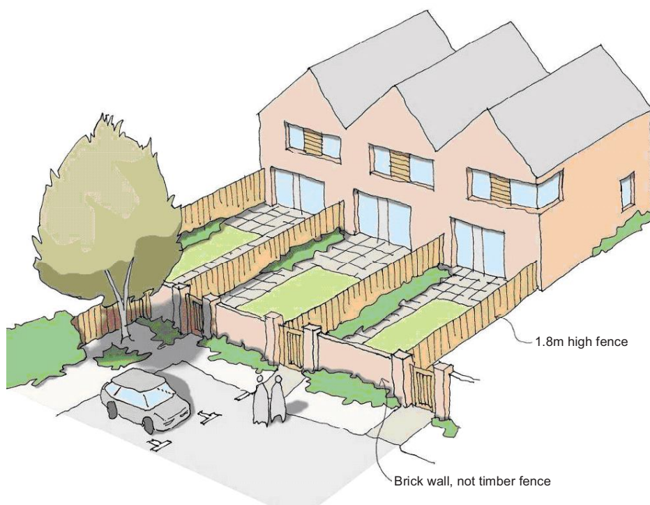
Figure 5.6: Appropriate boundary structures for rear private gardens
