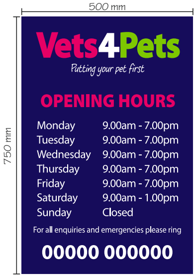
SIGN 2 FOLDED ALUMINIUM PANEL WITH VINYL DETAIL APPLIED TO THE FACE
