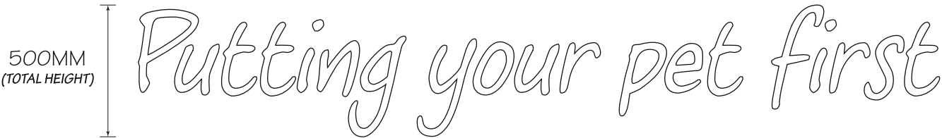
SIGN G STRAPLINE - ROUTER CUT WHITE FOAMEX LETTERS WITH NYLON LOCATORS.
