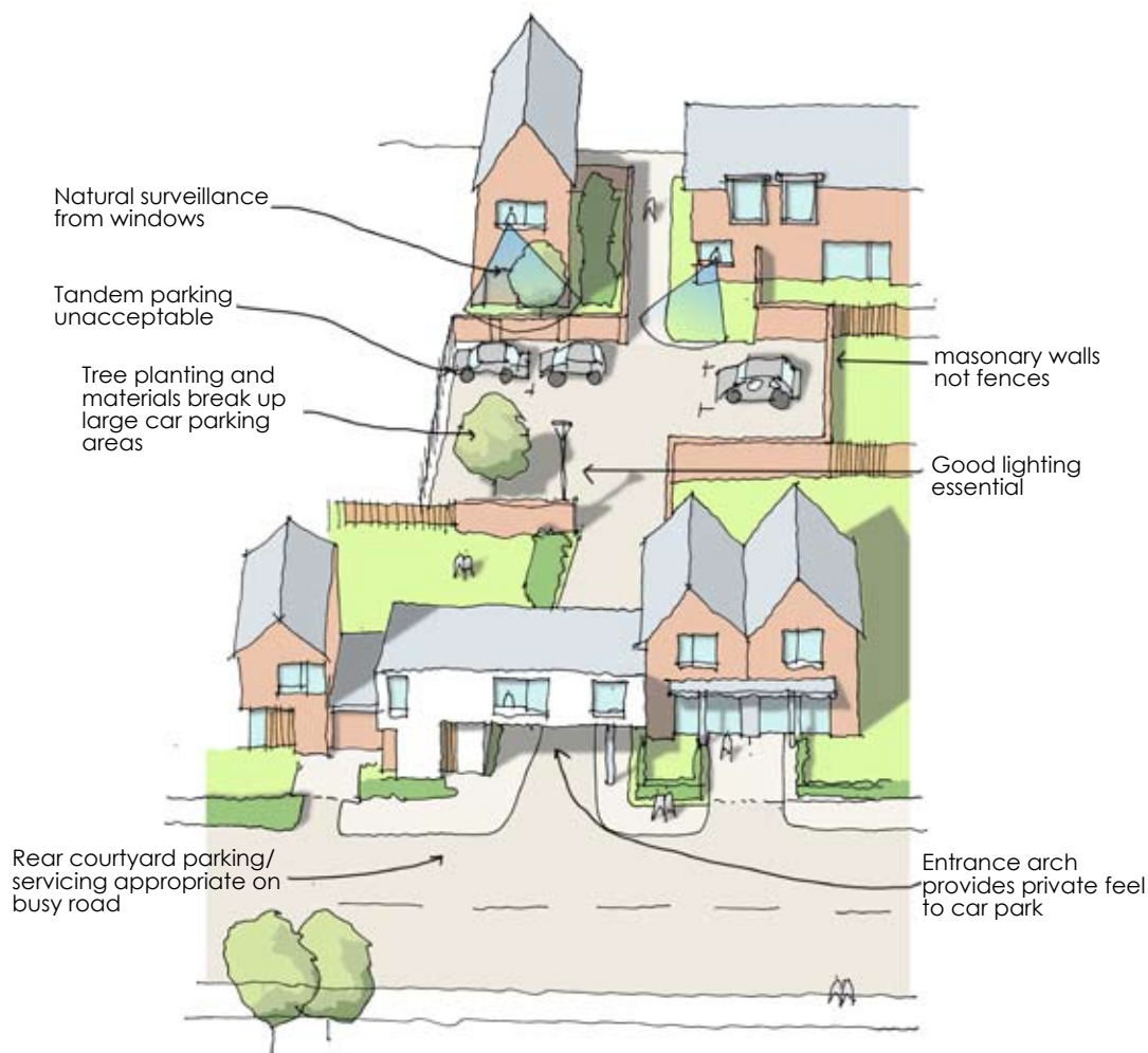
Fig.57: Rear court car parking
