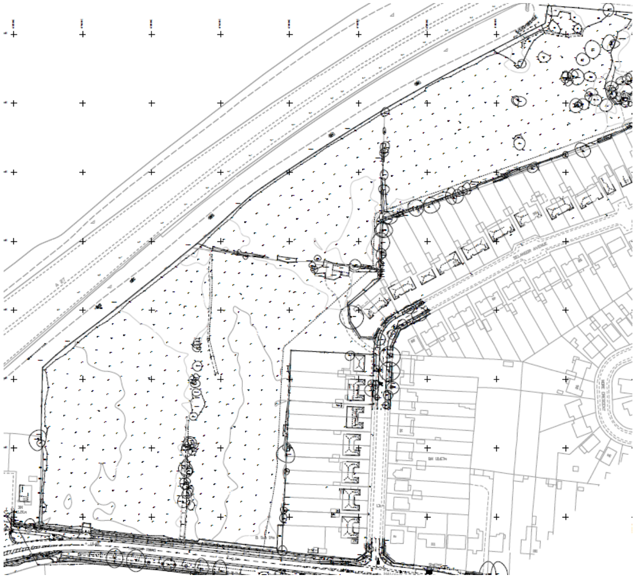
Figure 2 – Existing site topographical survey
