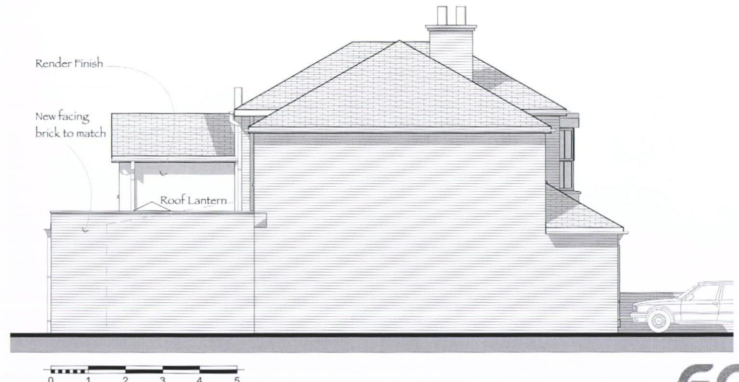
Proposed Side Elevation
