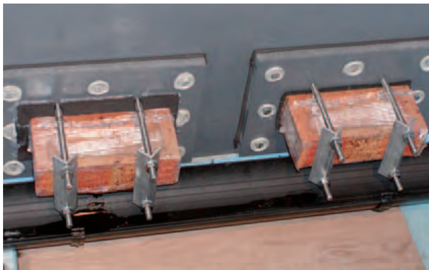
Figure 6.1 Pressed facing bricks being tested
