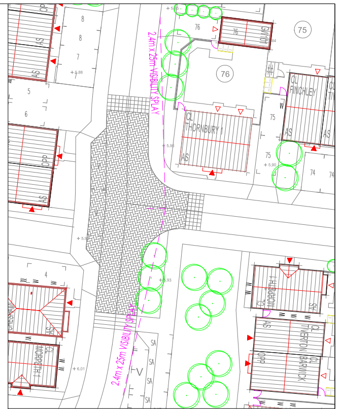
INSET 4 - 25m VISIBILITY SPLAY AT JUNCTION (1:500)
