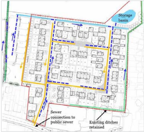
Surface Water Drainage
