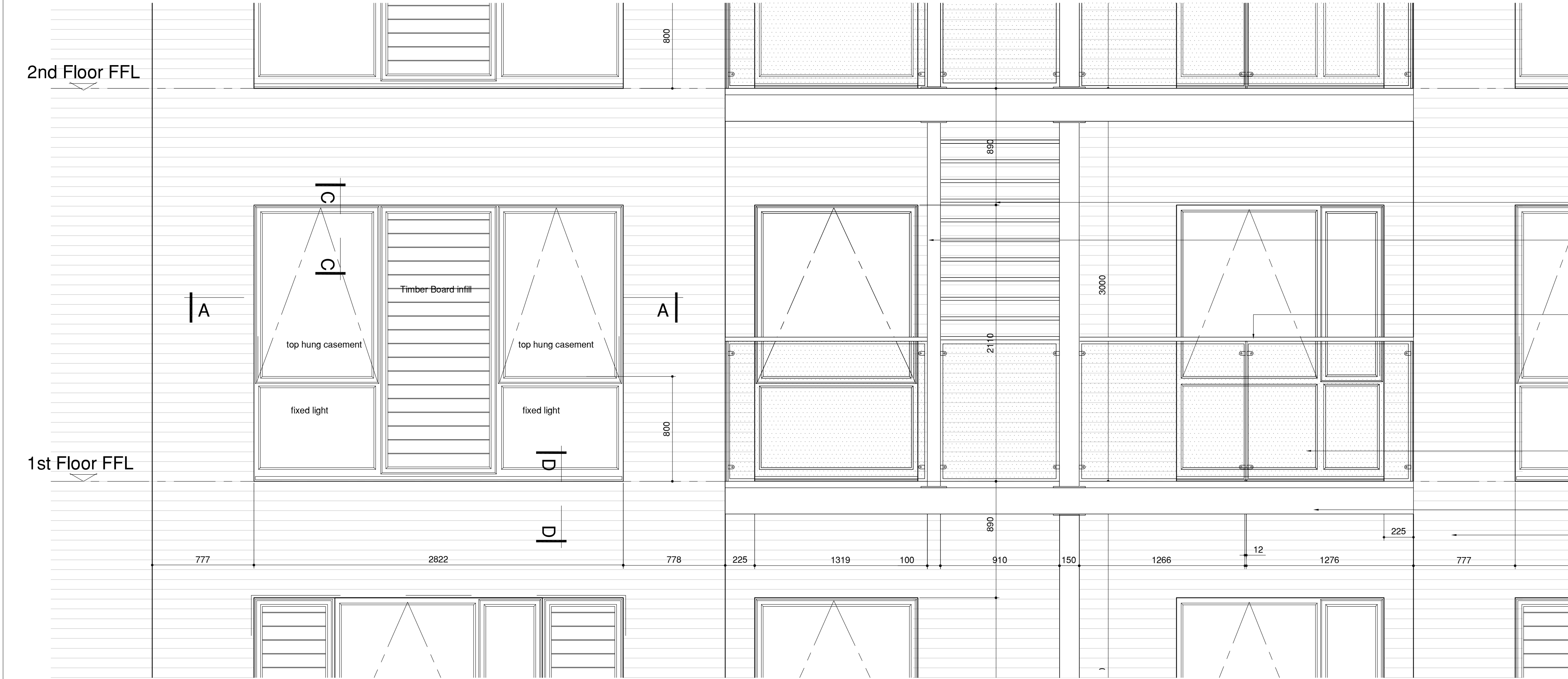
Detail Elevation at forward bay and balcony 1:20
