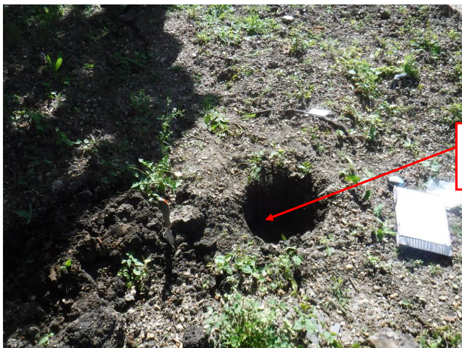
Sample hole through topsoil (Tp2)
