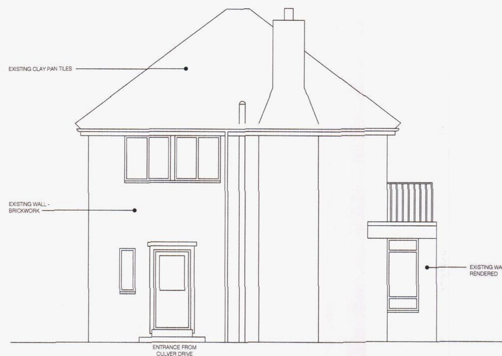
EXISTING WEST ELEVATION
