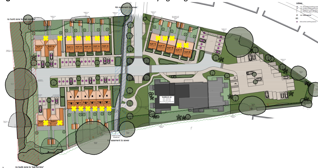
Figure 5. Location of sensor activated security lighting.
