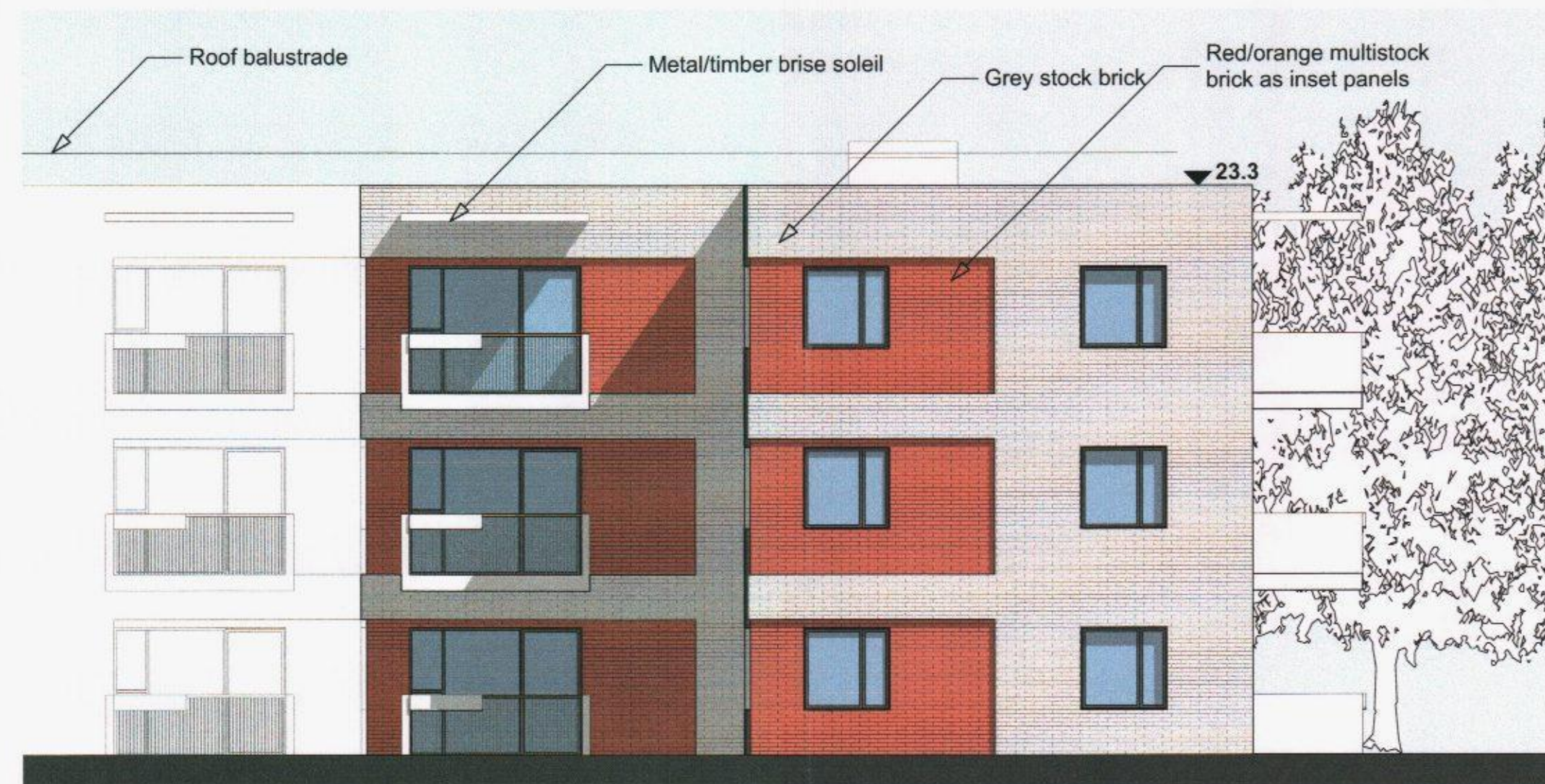
328 Supported Living North - South Elevation 1:100
