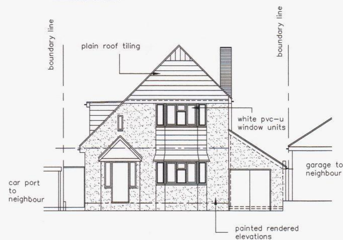
NORTH WEST ELEVATION
