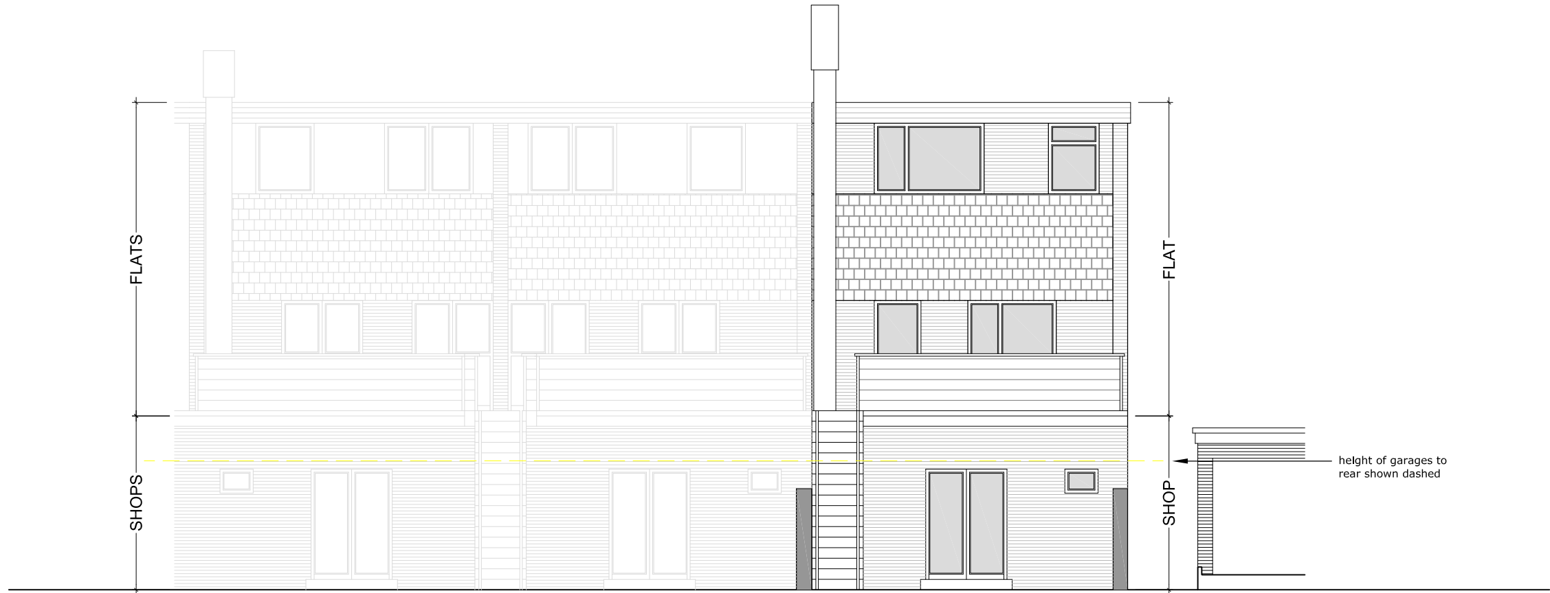
EXISTING REAR ELEVATION (D) - Adjacent to Garages, Rear of ground floor shops and upper level flats
