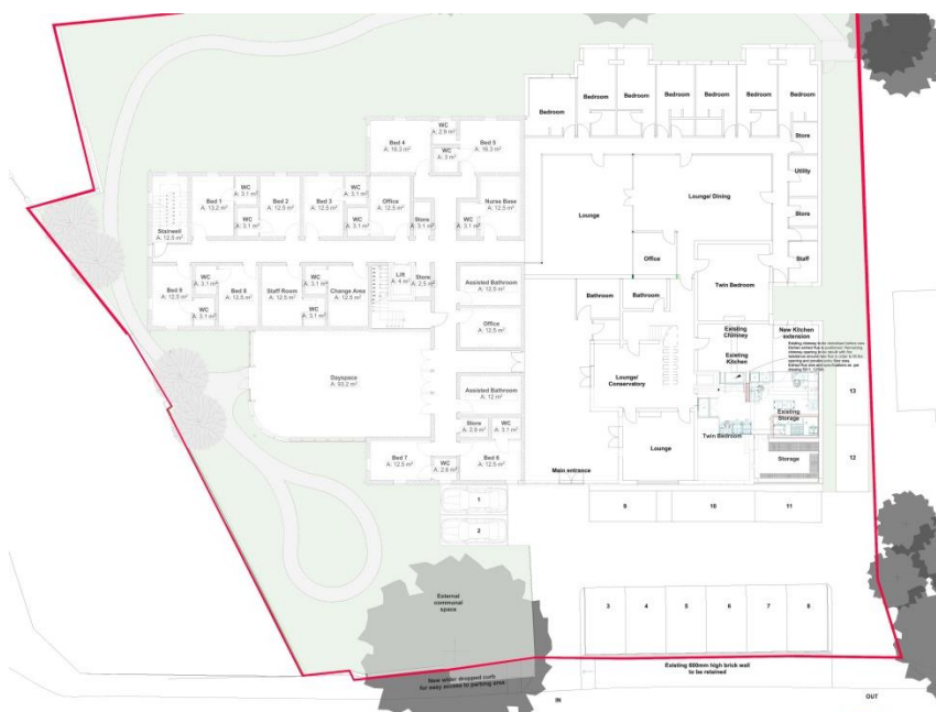
Fig. 1: Proposed ground floor plan
