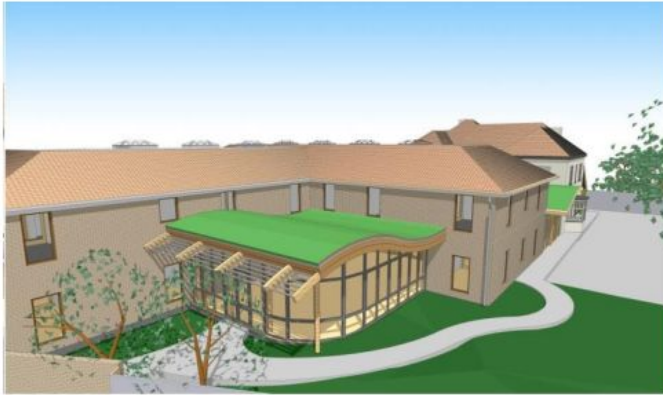
Fig.2: Proposed sunroom with green roof system
