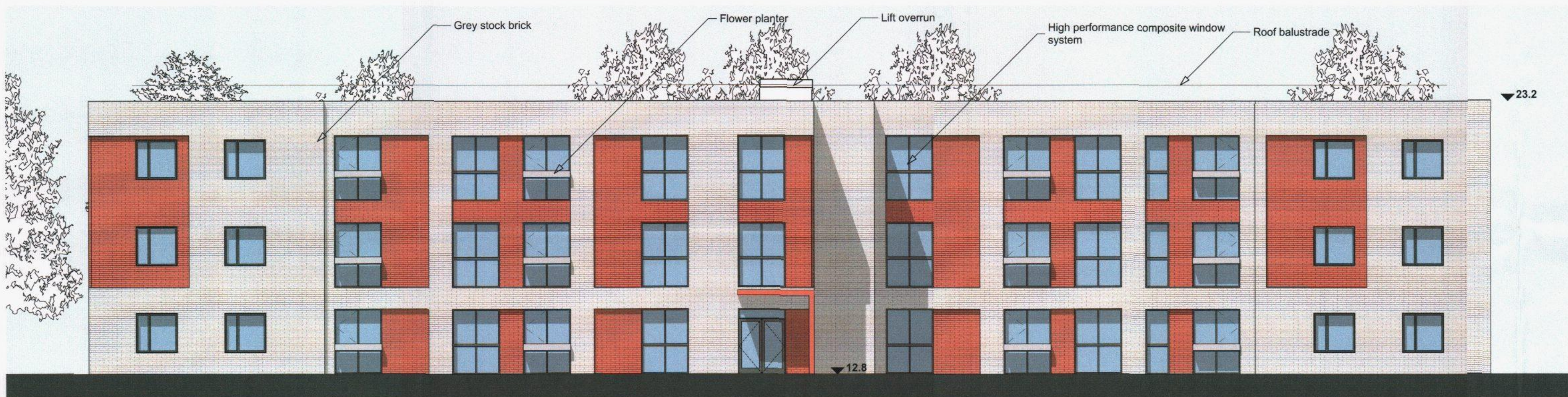
329 Supported Living South - West Elevation 1:100
