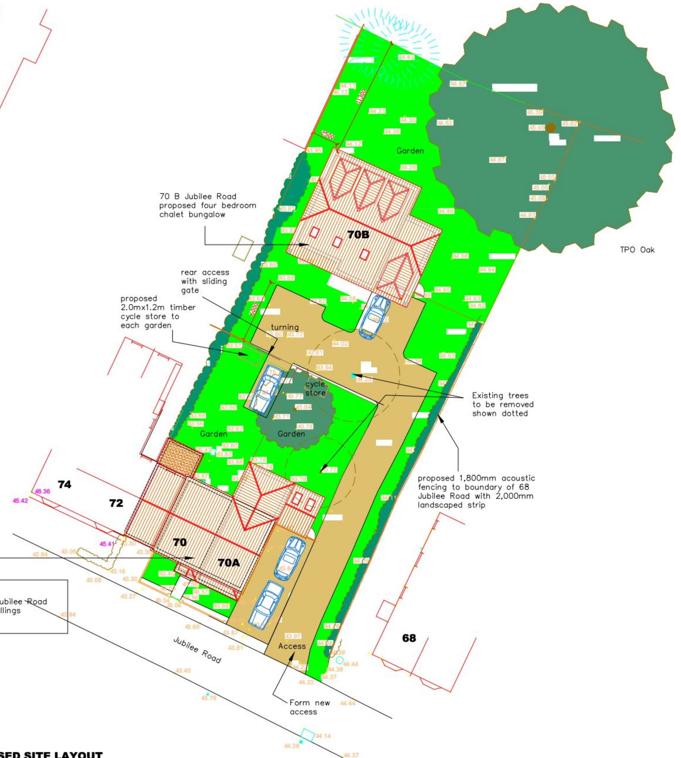
PROPOSED SITE LAYOUT SCALE 1 : 200
