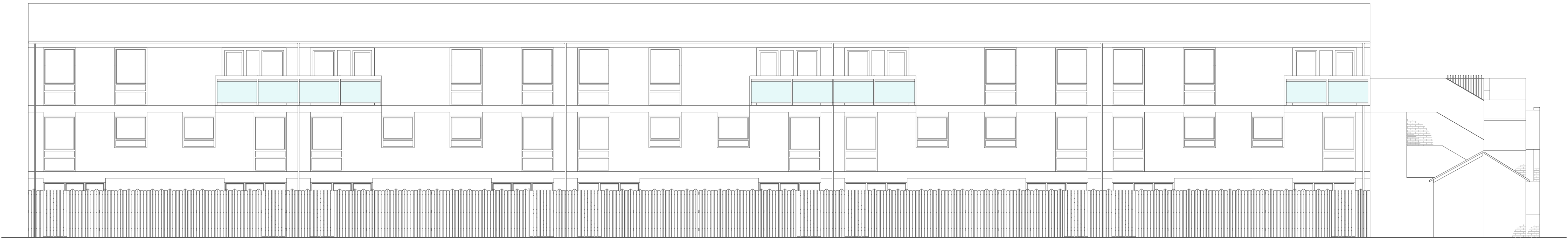
FULMER WALK 58-72 SOUTH ELEVATION - EXISTING GEORGIAN WIRED INFILL GLAZED PANELS TO BALCONIES
