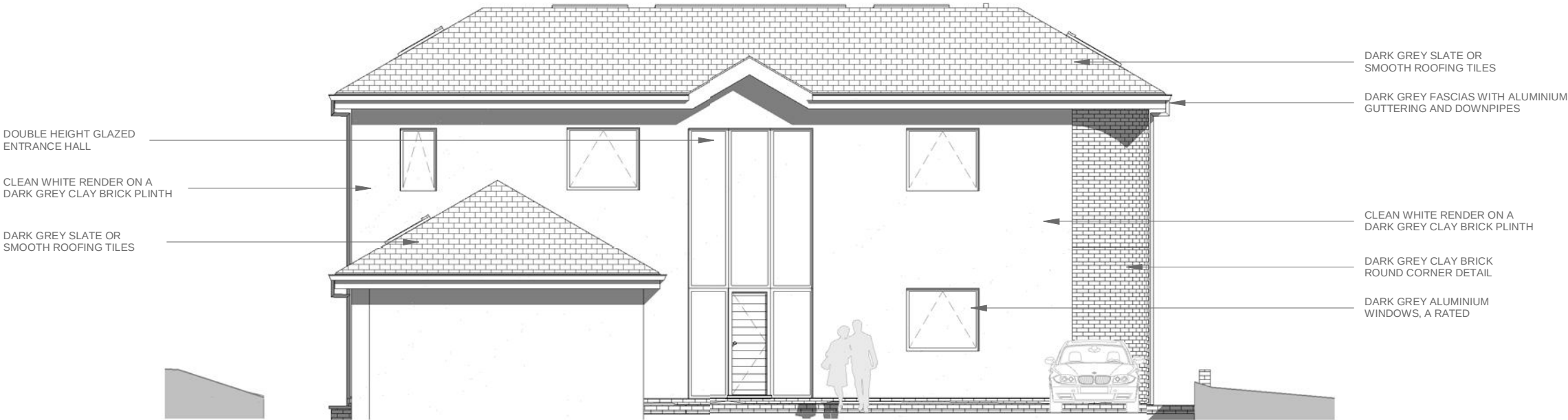
NORTH ELEVATION (FRONT) 1 : 100
