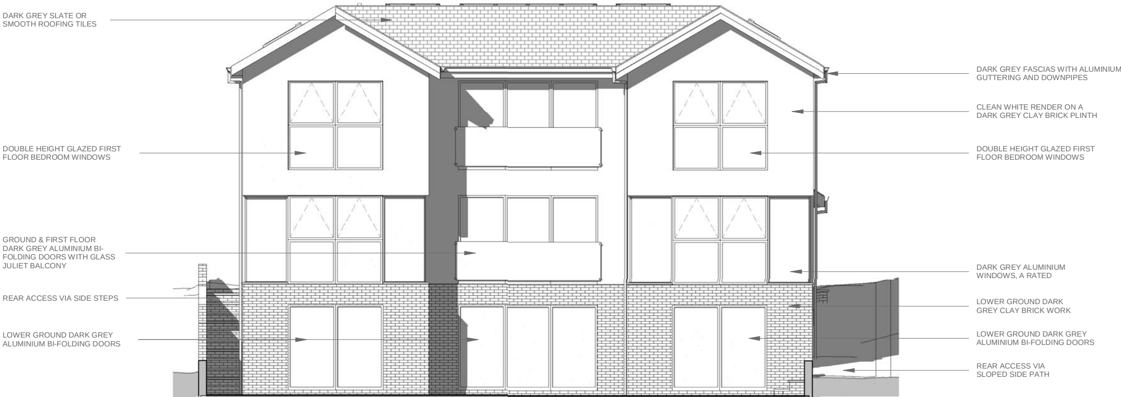
SOUTH ELEVATION (REAR) 1 : 100
