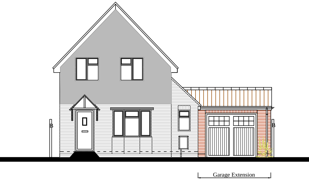
Front Elevation As Proposed Scale 1:100 (north west)
