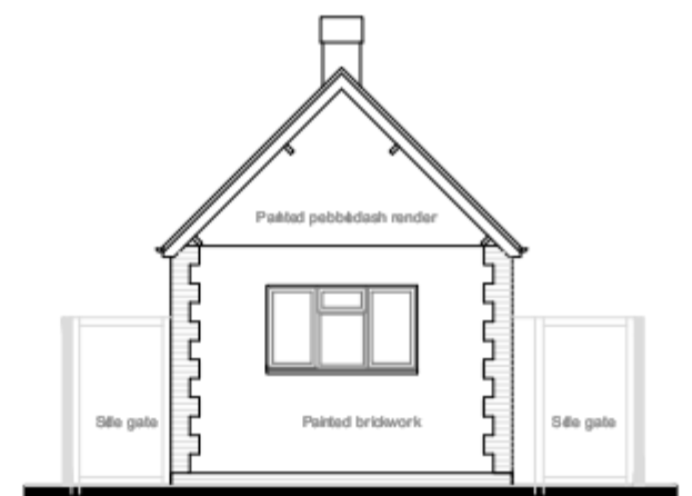
Side / front elevation - West
