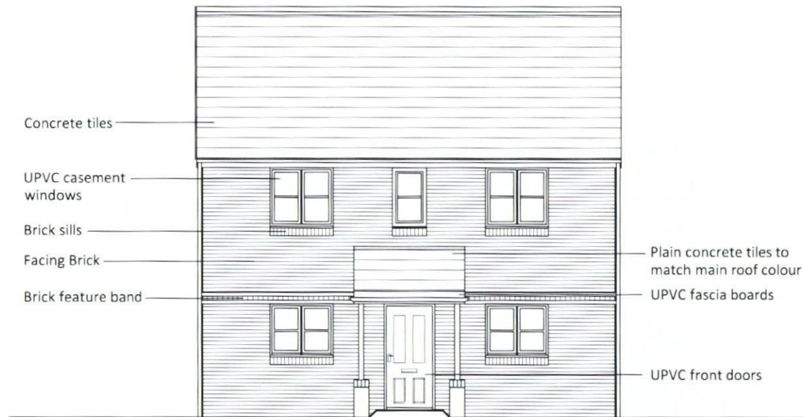
01 North Elevation (front) 54
