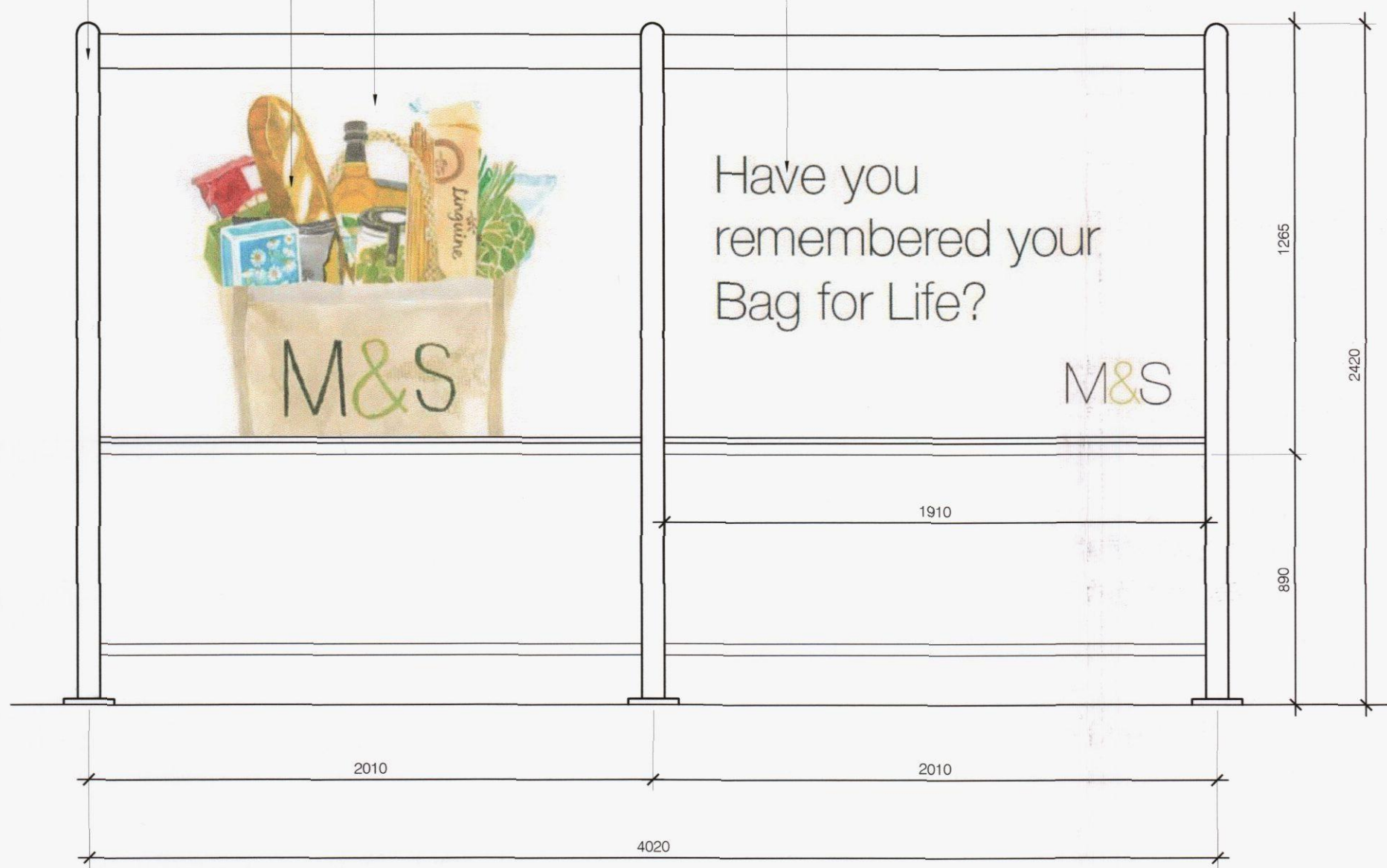
01 SIDE ELEVATION 406 1:20 TROLLEY BAY
