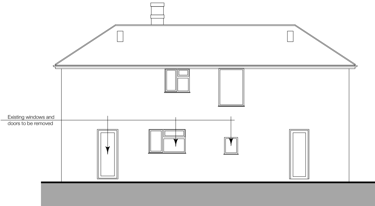
EXISTING NORTH ELEVATION 1:100
