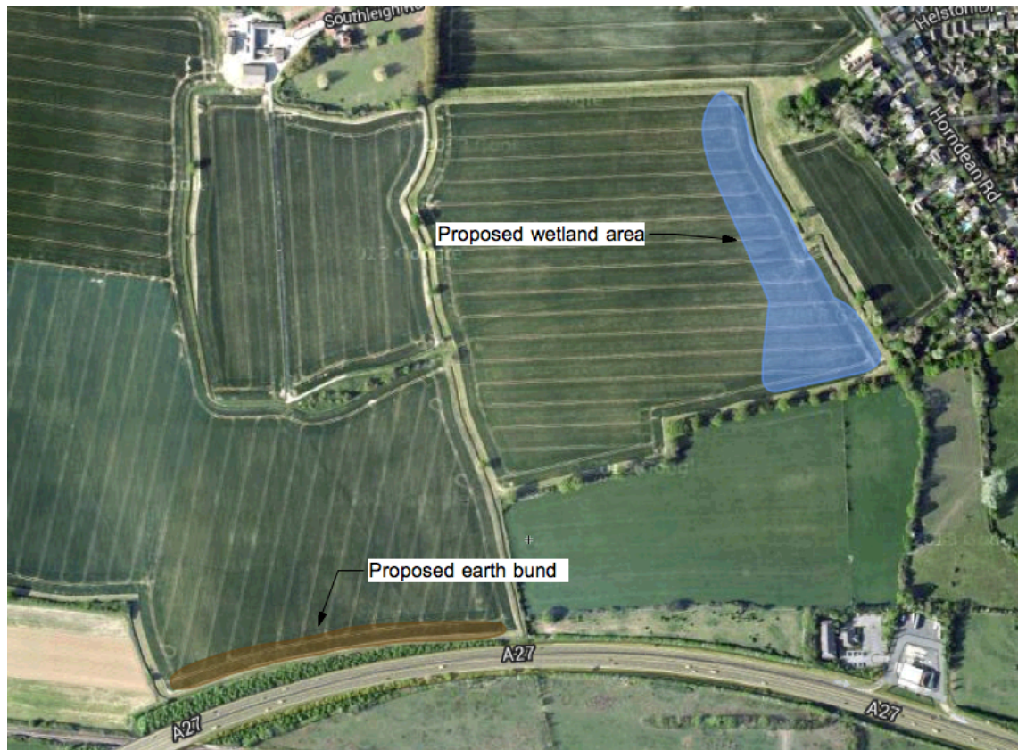
Picture 1 – An aerial picture of the site, with indicative illustrations of the proposed wetland site and associated bund.
