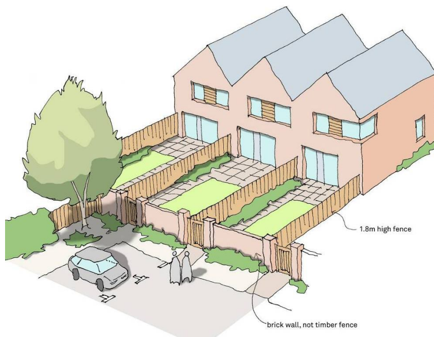
Figure 4.12: Appropriate boundary structures for rear private gardens
