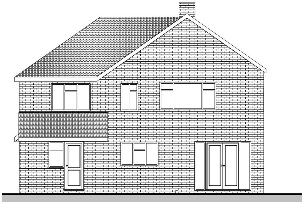
Existing Rear Elevation 1 : 100
