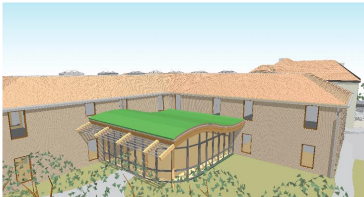
Fig.2: Proposed sunroom with green roof system
