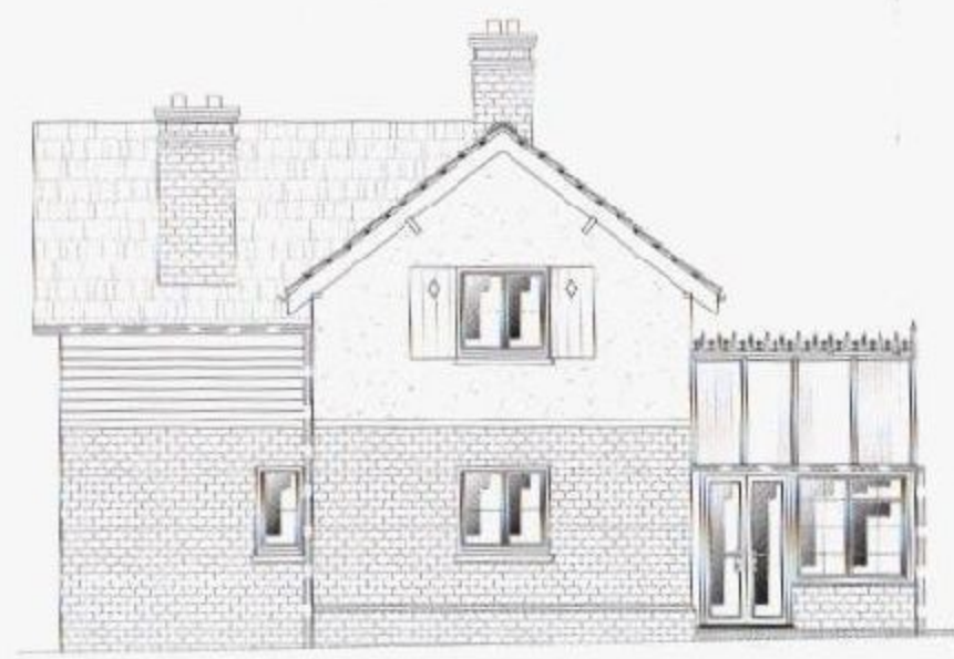
1 EXISTING SIDE ELEVATION 1:100
