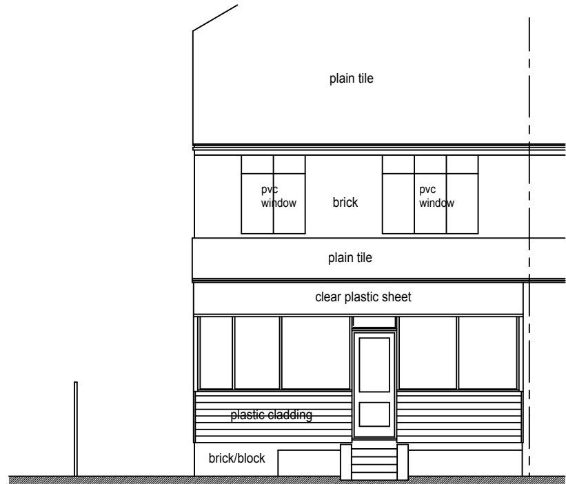
Existing North Elevation
