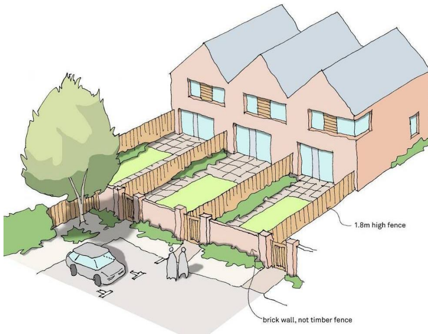
Figure 4.12: Appropriate boundary structures for rear private gardens
