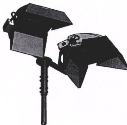
Figure 5 Proposed light fittings with front and rear cowls to minimise light spill
