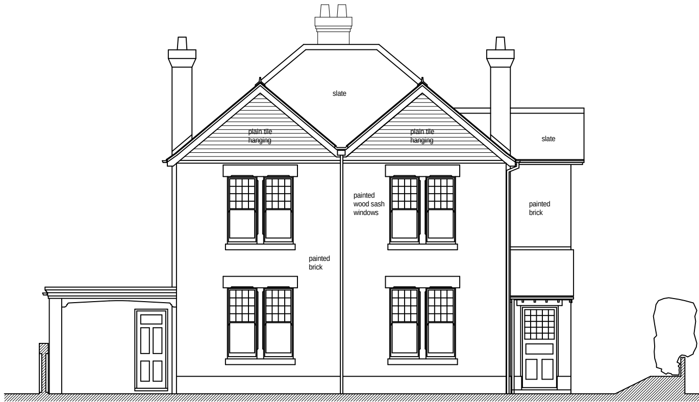
Existing North Elevation (to Hollow Lane)
