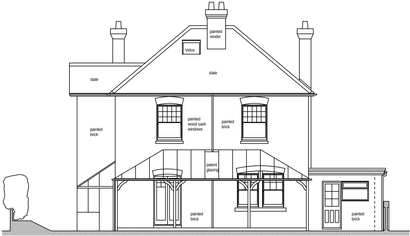
Existing South Elevation
