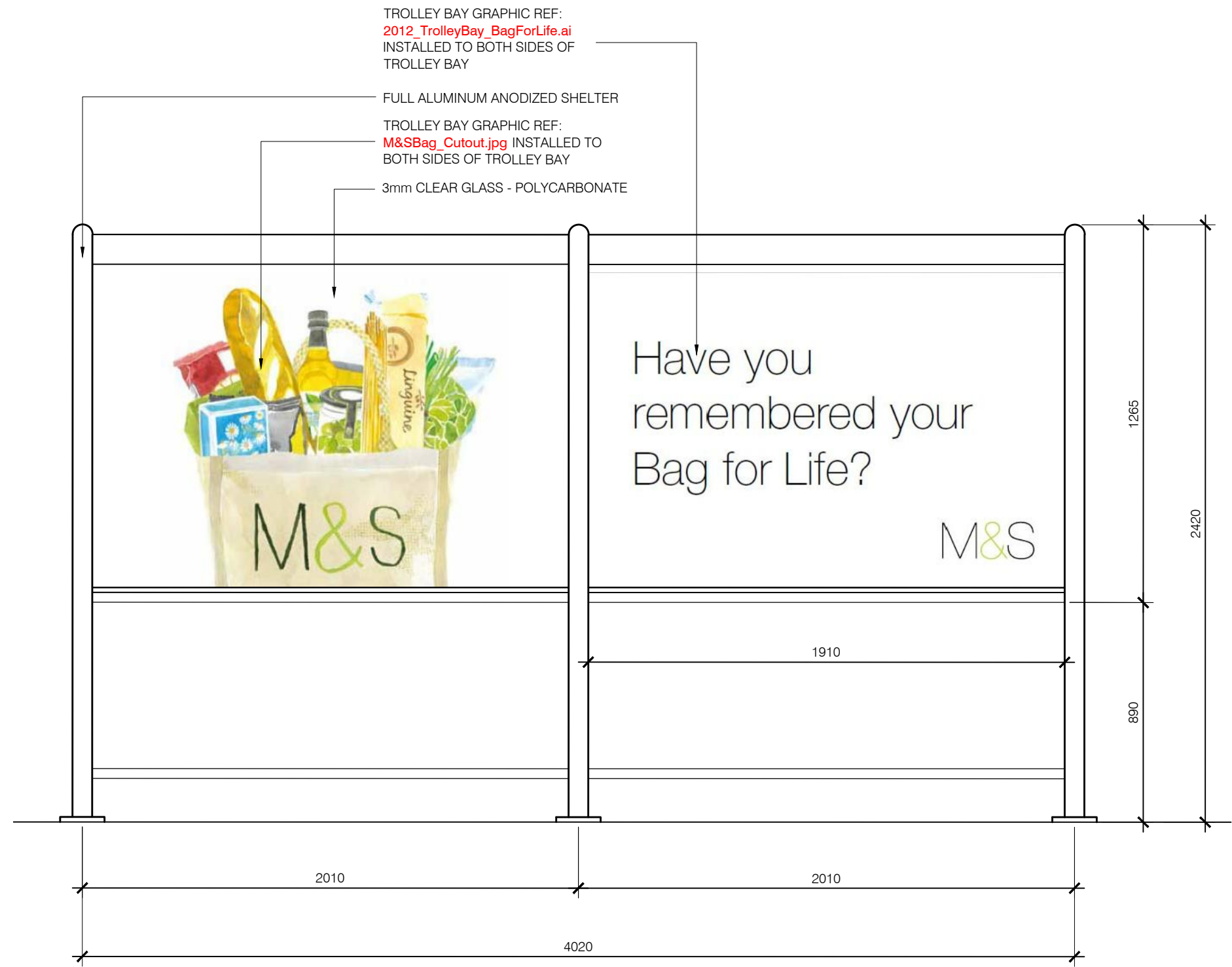
01 SIDE ELEVATION 406 1:20 TROLLEY BAY
