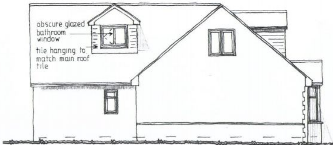
SIDE (SOUTH-WEST) ELEVATION
