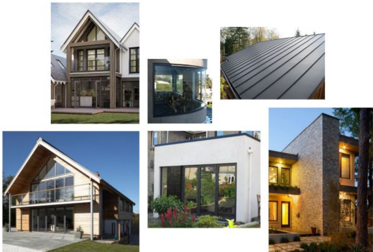
Image 7: Palette of materials (clockwise from top left); timber frame to balconies, curved glass to circular hall, standing seam zinc roof, natural stone walling, off-white render with grey windows, overhanging eaves.
