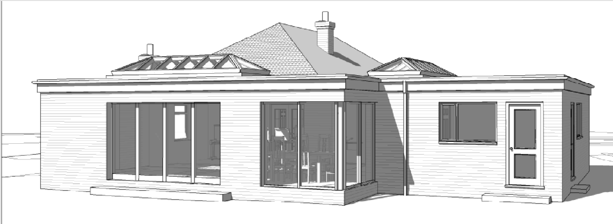
PROPOSED REAR ELEVATION SHOWING NEW EXTENSION
