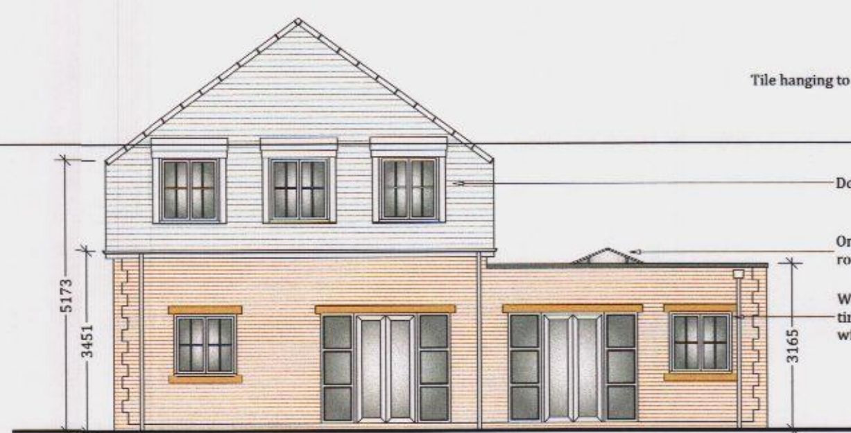
UNITS 3, 4 & 5 - REAR (EAST) ELEVATION 1:100
